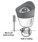
3. Adjust the camera to target the video location and tighten the camera bracket handle on the camera bracket.
